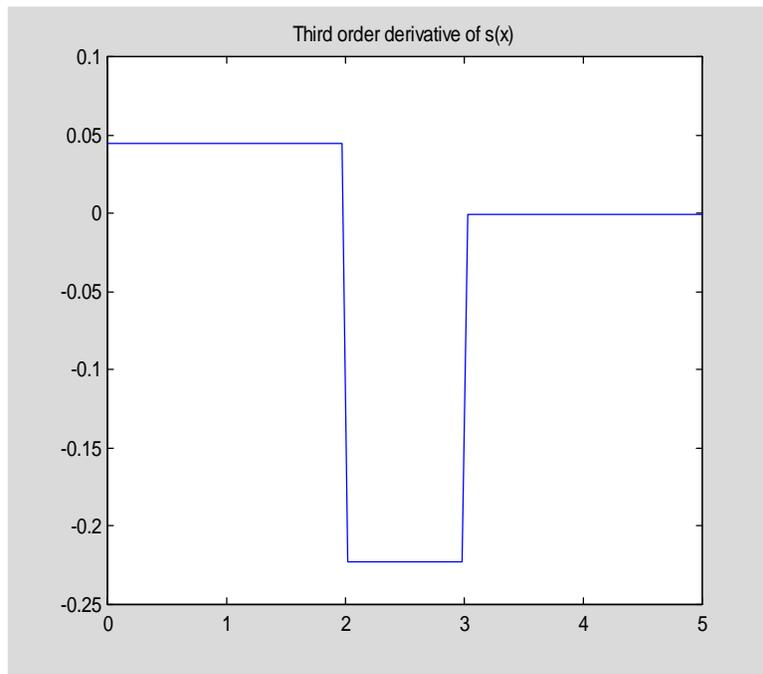
Note that  $s'''(x)$  is continuous at the breakpoints  $x_2 = 1$  and  $x_5 = 4$ . This is due to the fact that the not-a-knot boundary conditions were imposed on the spline interpolant.
