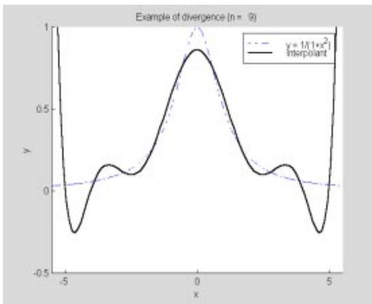
Divergence occurs at points that are close enough to the endpoints of the interval of interpolation `[-5, 5]`.
