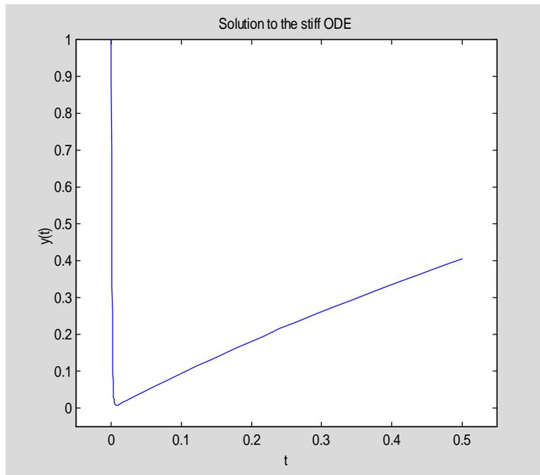
The exact solution to this problem is  $y(t) = \log(1+t) + \exp(-1000*t)$ . Try to plot this function on the interval `[-0.05, 0.5]`.
